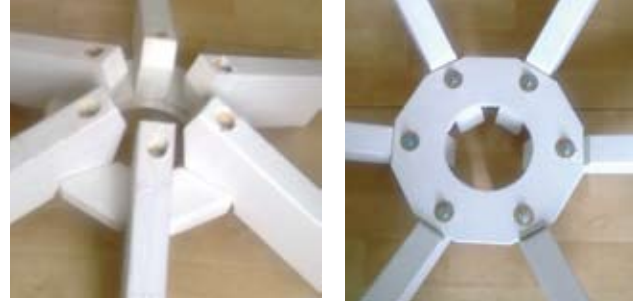
Picture of steel connecting plate above and beside, picture of plywood attachment used in hexagonal in the two above.
