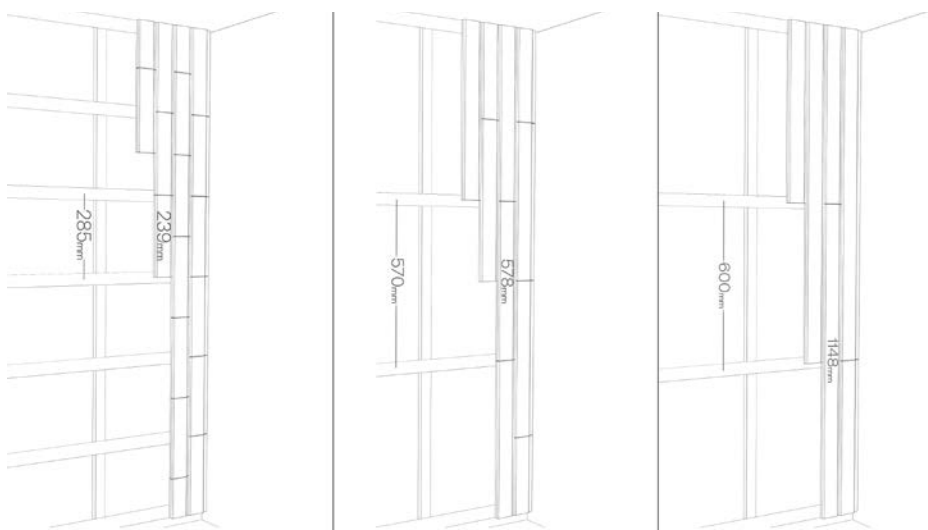
Tiles by Thermory panels vertical installation
